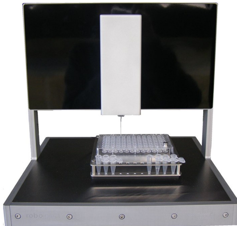
Figure 9. Picture of Roboinject setup as it was used for RNA injection of X. laevis oocytes. The picture was taken from the official Roboinject manual with kind permission from Multi Channel Systems MCS GmbH.
