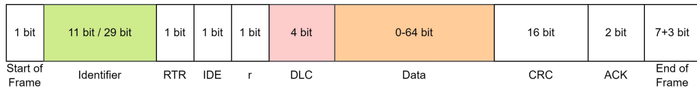
Figure A.1: Illustration of a complete CanBus frame. The green marked bits represent the frame identifier also used to prioritise messages. The red marked bits are the data length code (DLC) bits and the orange marked bits correspond to the data [81].
