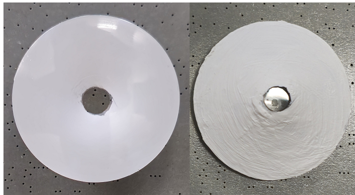
Figure 6.5: Example of a well painted light collector with an outer diameter of 25 mm. The paint was applied in a span of three days with each being a single thin layer. The inside (left hand side) and outside (right hand side) are homogeneous and no visible cracks can be seen.
