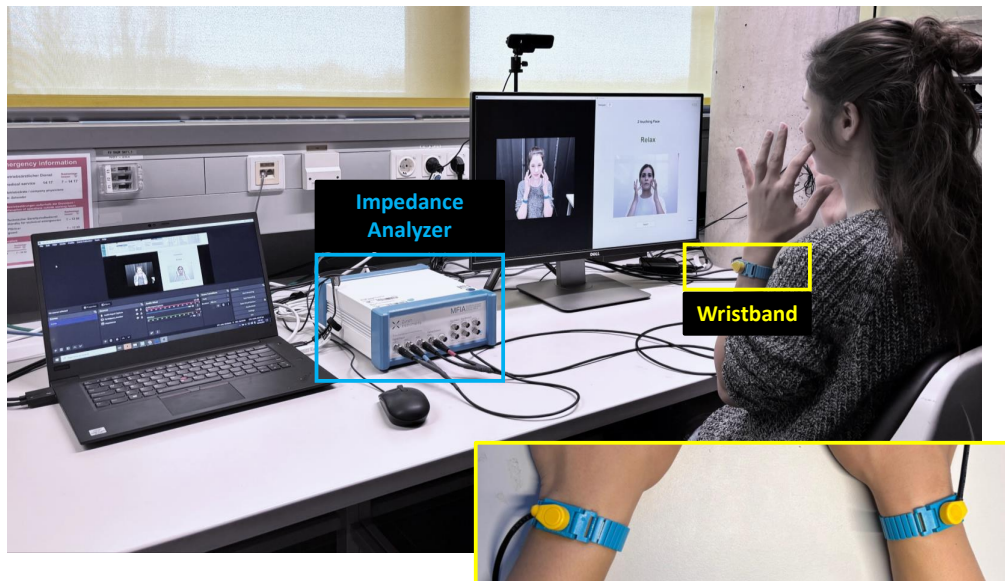
Figure 4.1: Experimental setup. The participant wears the wristbands on their left and right wrists. The electrodes in the wristbands are connected to the impedance analyzer through BNC cables. The screen shows the name and a mirrored image of the pose to be mimicked, a message that states whether the participant needs to hold the pose, and their own mirrored video stream captured with an external camera placed above the screen. The laptop computer records the data. The inset shows a top view of both wristbands.
