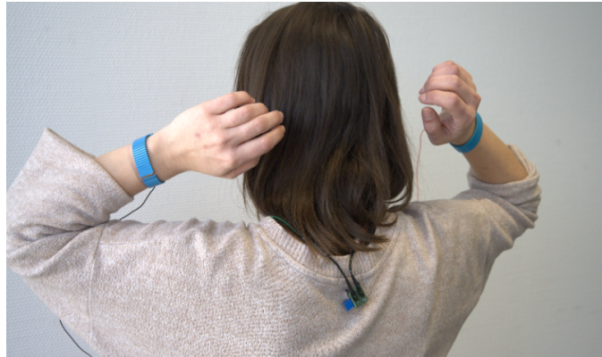
Figure 5.2: Wearable setup. We created a miniaturized sensor that consists of a processor, shown here attached to the wearer’s shirt, and two electrodes embedded in the blue bracelets on their wrists. All components can be hidden beneath clothing.
