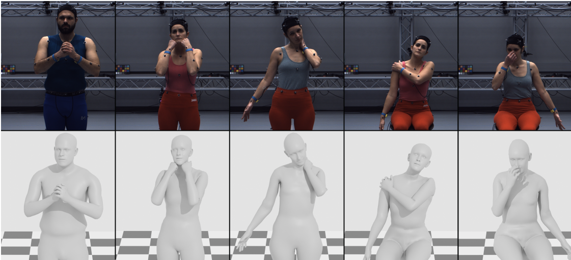
Figure 5.4: Sample contacts that cause a significant change in the bioimpedance of the user. Any self-contact (direct on skin or through body hair) greatly impacts the wrist-to-wrist bioimpedance signal. The videos from which these images were taken and their ground-truth SMPL-X meshes are part of our newly collected dataset.
