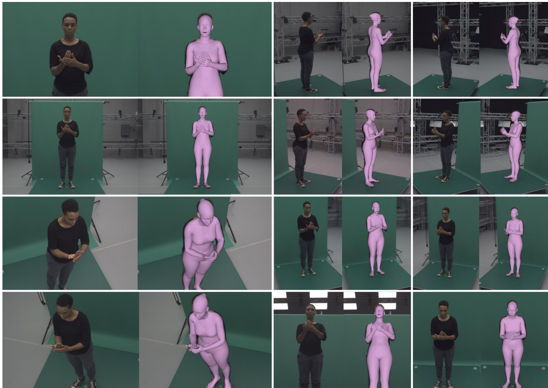
Figure 3.10: Multi-view setup with the 12 synchronized RGB cameras and their SGNify reconstruction.
