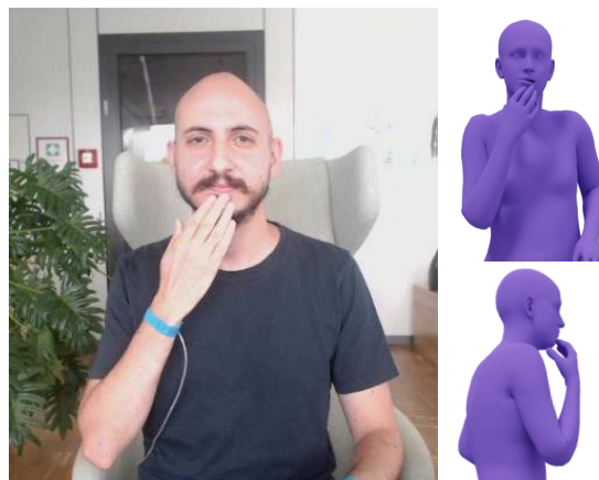
Figure 6.1: THANKS (ASL) in the original video and reconstructed by SGNify with BioTUCH. Both frontal and side views demonstrate effective reconstruction, with the hand contacting the face.
