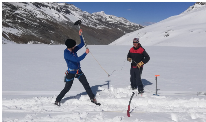
Figure 1.11: Performing reflection seismics to measure the thickness of Hintereisferner (Photo taken by Inka Koch).
