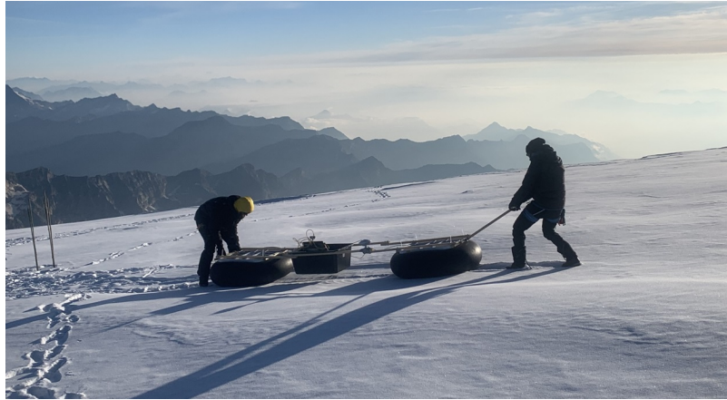
Figure 1.10: Phase-coherent radar profiling in mountainous terrain with mobile pRES on Colle Gnifetti (Photo taken by Reinhard Drews).
