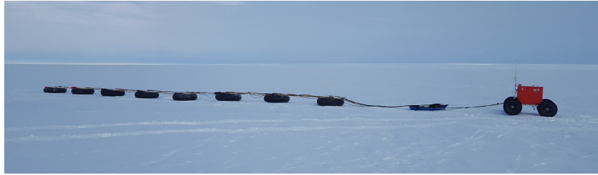
Figure 1.12: Mobile multiple-input multiple-output pRES survey for SAR processing of the englacial and basal structure of Ekström ice shelf acquired using the autonomous rover presented by Ershadi et al. (2024).
