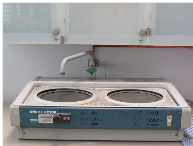
Figure A.5: A view graph of the grinding machine (KNUTH-ROTOR), with two SiC plates of different grit size.
