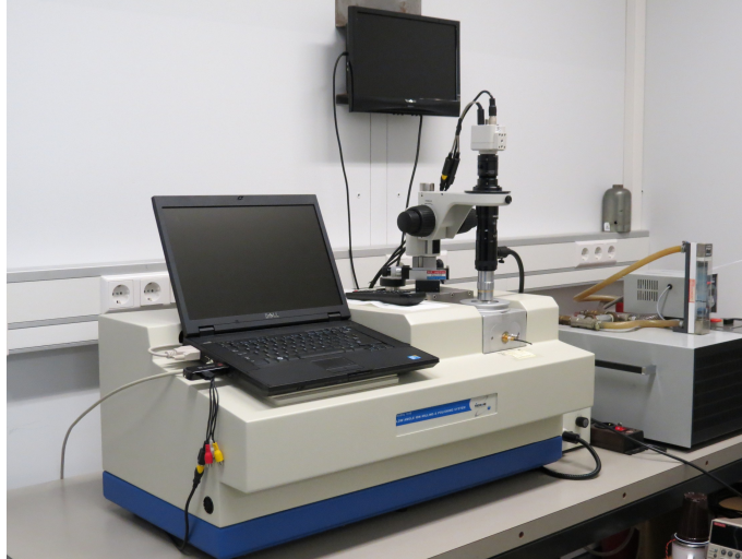
Figure 2.6: A view graph of Fischione 1010 low-angle ion etching machine.
