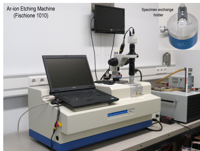
Figure A.1: A view graph of the Ar + ion etching machine (Fischione 1010).
